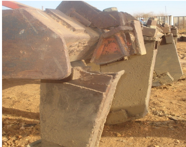
Figure 8: Lack of a protection device damaged a shank of a chisel plow
