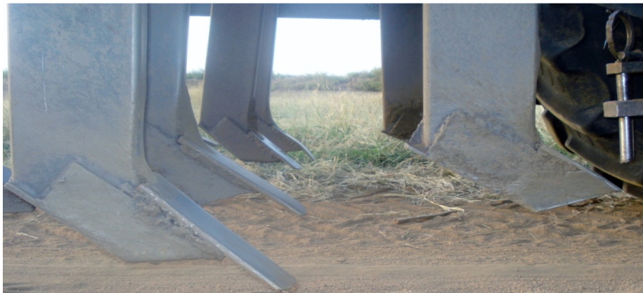
Figure 9: A chisel plow with front and rear shanks of different lift angles
