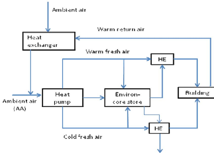
**Appendix (5) Flow chart of combined heating and cooling with air-source heat pump and energy recovery from return air in combination with Environ-core thermal storage**
