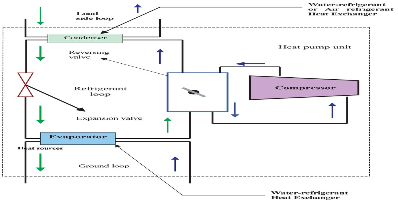
Figure 9. Schematic of GSHP system (heating mode operation)
