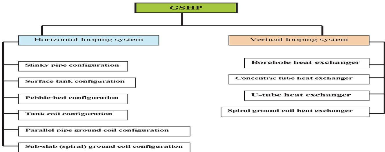
Figure 8. Common types of ground-loop heat exchangers
